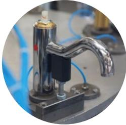
Cycle Testing (3X ASME STD)
